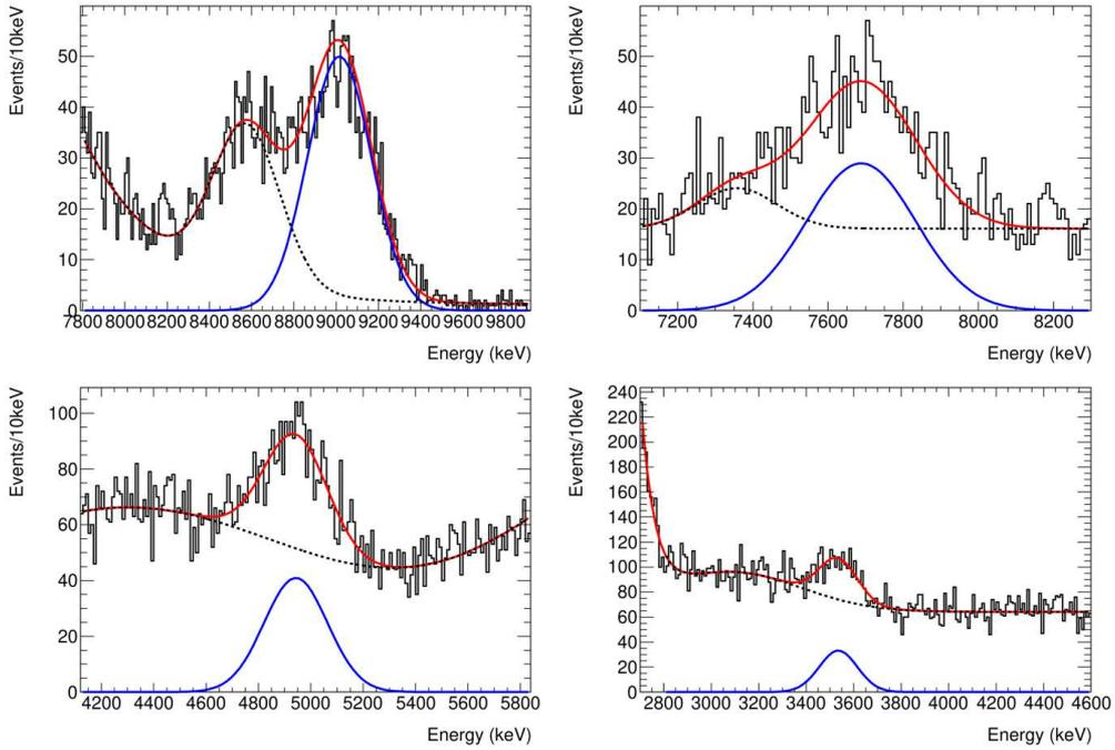
Figure 5: Fitting results for 8,998 keV of  $^{58}\text{Ni}$  (top left), 7,631 + 7,645 keV of  $^{56}\text{Fe}$  (top right), 4,934 keV of  $^{28}\text{Si}$  (bottom left), and 3,539 keV of  $^{28}\text{Si}$  (bottom right), respectively. The red line shows the fitting results, the black dashed line shows the background, and the blue line represents the signal
