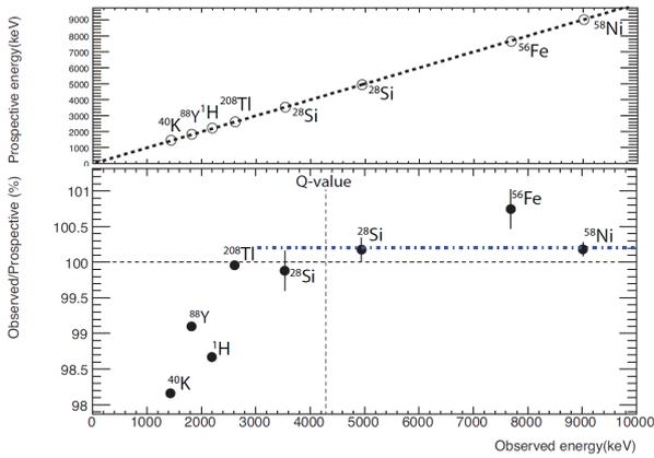
Figure 6: The top image shows prospective energy vs observed energy. Each point corresponds to  $\gamma$ -ray peak energy measured by calibration or background run. The bottom image shows energy deviation for CANDLES as a function of observed energy. Blue dash-dot line is an average obtained from four new calibration points. Good linearity of energy response within 0.3 % was obtained in the region of interest by this work. Error bar shows only statistical error.
