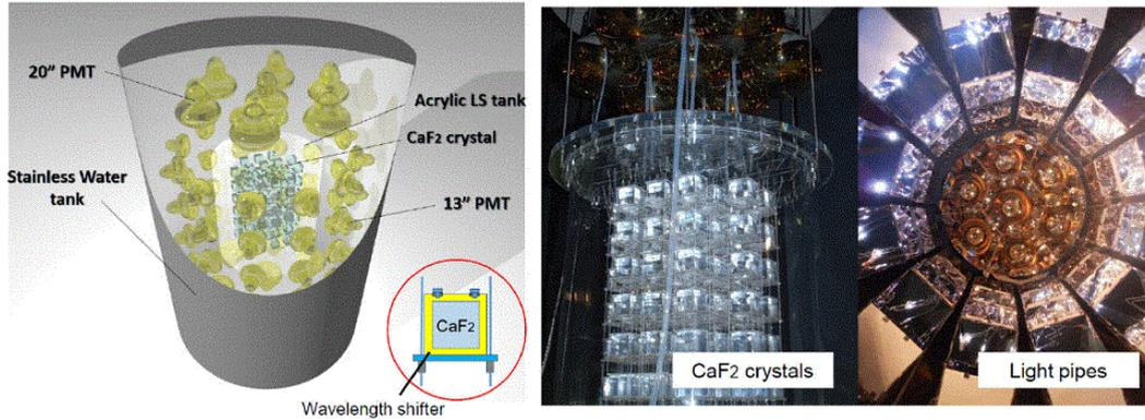
Figure 1: The figure on the left presents a schematic view of the CANDLES III detector. The stainless steel tank has a 3-m diameter  $\times$  and a 4-m height. The acrylic tank is 1.4 m in diameter  $\times$  and has a height of 1.4 m. The size of the  $\text{CaF}_2$  crystal is  $10^3 \text{ cm}^3$  cubic. Light pipes have been omitted from the figure for better visibility. Two images on the right show the CANDLES  $\text{CaF}_2$  crystal array and light pipes seen from above the tank.
