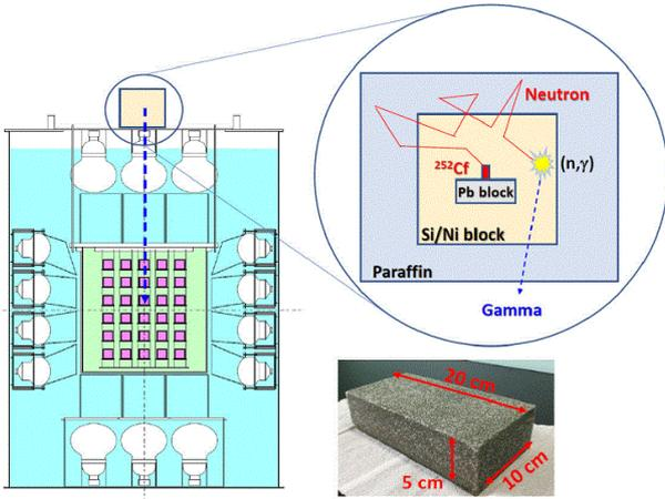
Figure 3: Schematic view of the calibration system. Si and Ni blocks were set on top of the CANDLES detector. Neutrons emitted from  $^{252}\text{Cf}$  were moderated by collision on hydrogen atoms and finally captured by  $^{28}\text{Si}$  or  $^{58}\text{Ni}$  nuclei, followed by  $\gamma$ -ray emission. The bottom right image shows a Si block sized 20 cm  $\times$  10 cm  $\times$  5 cm.
