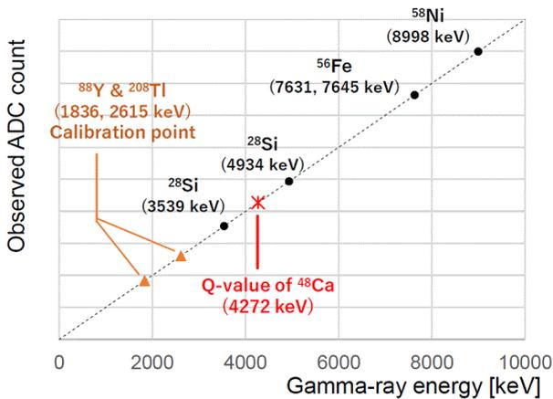
Figure 2: Conceptual plot for the CANDLES energy calibration. The cross marker shows the Q-value of  $^{48}\text{Ca}$ ; the triangle indicates the current calibration point at 1,836 keV for  $^{88}\text{Y}$  and 2,615 keV for  $^{208}\text{Tl}$ . The black circle shows the new calibration point added by this paper.
