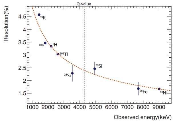
Figure 7: Energy resolution ( $\sigma$ ) for CANDLES as a function of observed energy. The circle marker indicates  $\gamma$ -ray observed in CANDLES by calibration and background run. Single exponential function indicated good fit with the data up to 9 MeV (dashed line);  $^{40}\text{K}$  near the detector threshold was removed from fitting points. The error bar indicates only statistical error.
