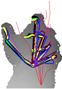
Fig. 2. Visualization of ground-truth hand pose and poses with varying level of MJEs, < 5mm , < 10mm , < 20mm , < 30mm , < 40mm , < 60mm . MJE (mm) of the visualized poses are 1.75, 6.88, 13.94, 15.32, 35.67, 52.15, respectively. Best viewed in color.
