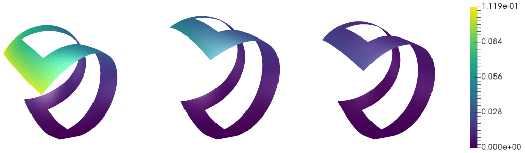
FIGURE 3. Numerical equilibrium states of the O-shaped plate in Section 7.2 for the triangulations \mathcal{T}_\ell , \ell = 3, 4, 5 with corresponding energies of 0.8869, 1.444 and 2.026 (left to right) colored by the magnitude of |\nabla y_h^k|^\top \nabla y_h^k - I_2| .
