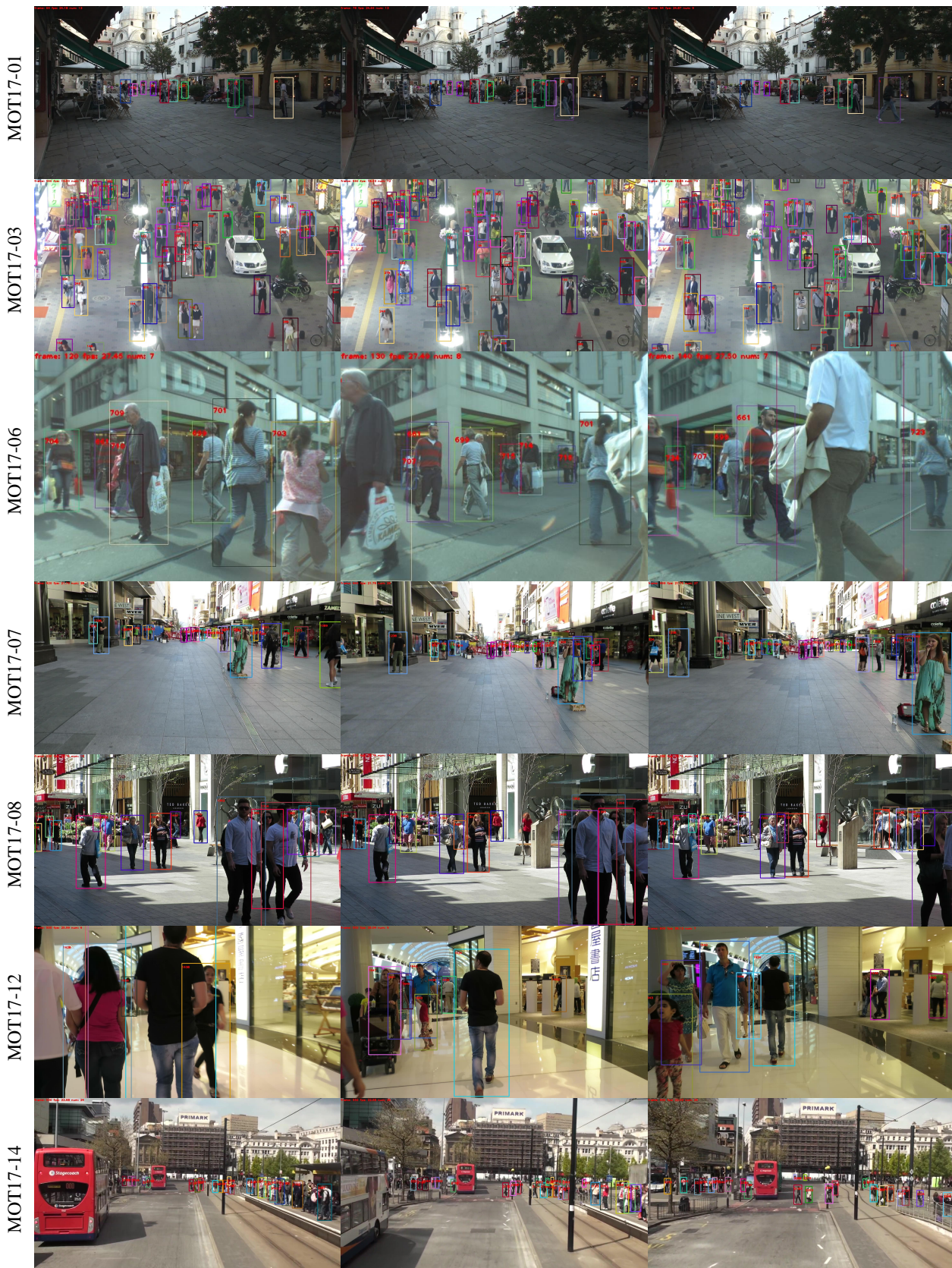
Fig. 5 Example tracking results of our method on the test set of MOT17. Each row shows the results of sampled frames in chronological order of a video sequence. Bounding boxes and identities are marked in the images. Bounding boxes with different colors represent different identities. Best viewed in color.
