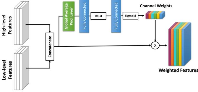
Fig. 2. Illustration of the attention mechanism in which an SE Block [25] is adopted on concatenated multi-level features
