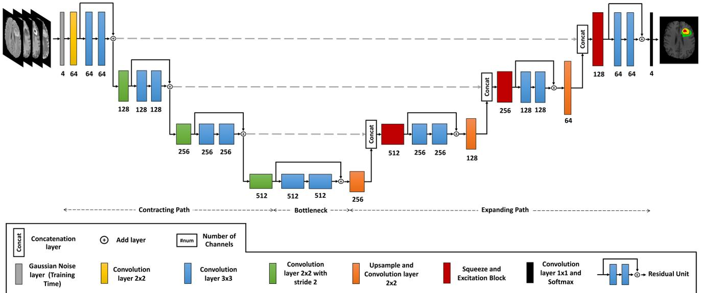
Fig. 1. The architecture of our proposed network which is based on UNet architecture.
