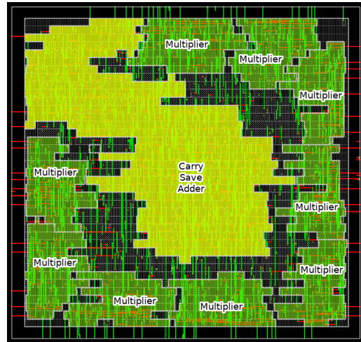
Figure 1: Our 3 \times 3 kernel 8-bit processing engine (PE) layout using the TSMC 28nm technology. The carry-save adder can fit 12-bit numbers, which is large enough to store the output of the convolution.
