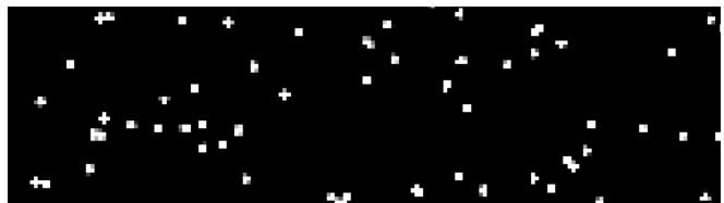
FIG. 4. Section of a Skipper-CCD image after exposing it to the X-rays emitted by the ^{55}\text{Fe} radioactive source where different cluster size can be identified.
