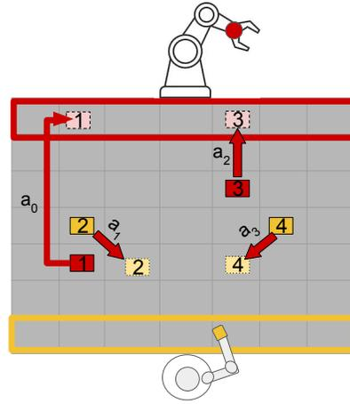
Fig. 2. An example board configuration consisting of blocks (1 – 4) for the robot (red) and the human (yellow). Robot actions ( $a_{0-3}$ ) are depicted by the arrows.  $a_0, a_2$  are *task-oriented* actions while  $a_1, a_3$  are *supportive* and  $a_1$  is a more useful *supportive* action because it reduces potential interference when reaching for block 1.
