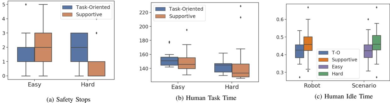
Fig. 6. Objective Measures. Box-and-whisker plots of the (a) number of safety stops; (b) time taken by the human to complete the task; and (c) the proportion of idle time spent by the human. Note, T-O refers to the *task-oriented* robot.
