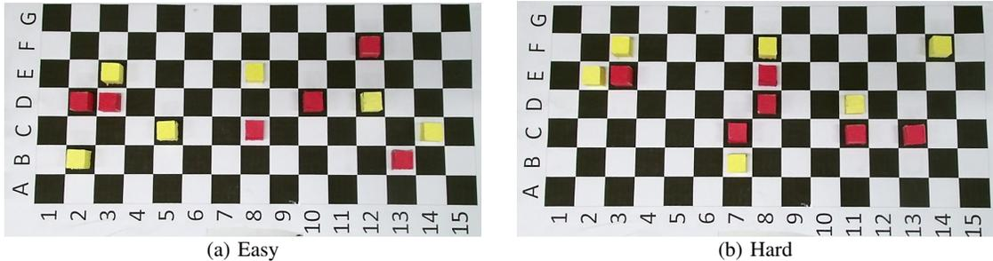
Fig. 4. Layout of the *easy* (left) and *hard* (right) block configurations, viewed so the human is seated below row A. The human places yellow blocks on the numbers below row A, whereas the robot is across the table and placing red blocks in Row G. The difficulty is due to the conflict caused by the robot and human reaching for the same space. This conflict exists more in (b) since most of the yellow blocks are in front of the robot’s.
