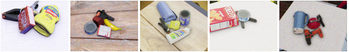
Fig. 3. Scenes generated by our physics-based arrangement engine. Object meshes are taken from the YCB Object set. Background images are randomly selected from an Internet image search with keywords “table surface”.
