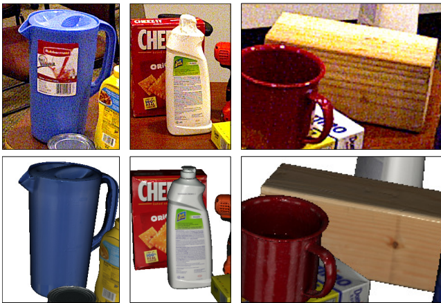
Fig. 6. Deviations of the real objects from their meshes: The top row shows crops of YCB-Video test frames, the bottom row their corresponding renders. The pitcher has a sticker on it, the cleaner bottle is wrapped with tape, and the wood block seems to have entirely different texture and surface finish. Furthermore, the mesh textures exhibit artifacts from the scanning process, such as the vertical reflection stripes on the cup.
