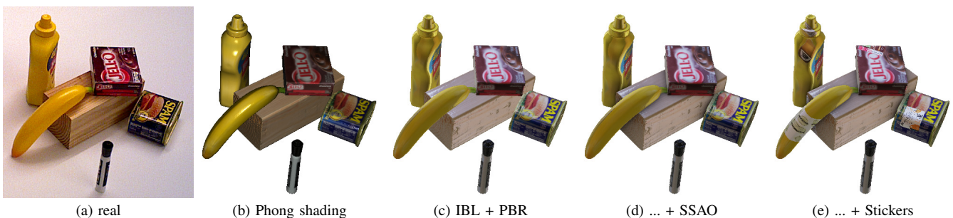
Fig. 4. Rendering extensions. For comparison, a real training image from the YCB-Video dataset is shown in (a). The other images show the effect of the discussed rendering extensions on a synthetic scene rendered with the same poses. Note that material settings for PBR (d) are randomized—which is why the mustard bottle looks metallic.
