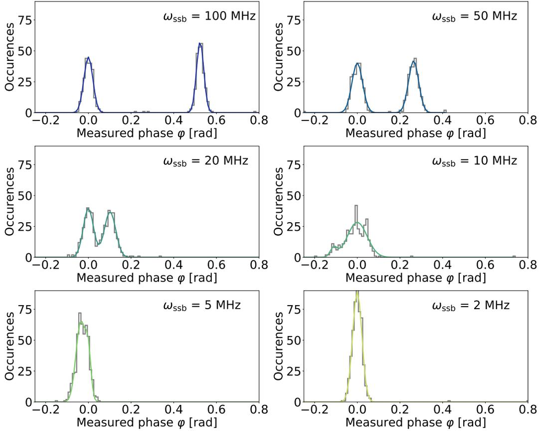
Figure 11. Reaction time jitter with synchronization unit: Histograms of the extracted iSWAP phases  $\varphi$  for slave AWG sideband frequencies of  $\omega_{sb}/2\pi = 100, 50, 20, 10, 5, 2$  MHz measured with  $M = 500$  repetitions.
