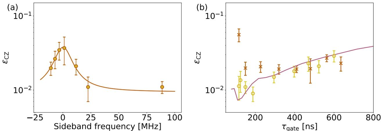
Figure 12. (a) Error per gate  $\epsilon_{CZ}$  of a CZ gate measured as a function of the sideband frequency. Solid line is a fit to a Lorentzian function with a sigma of 17 MHz. (b) Error per gate  $\epsilon_{CZ}$  as function of the gate length  $\tau_{\text{gate}}$  for a sideband frequency of 5 MHz (crosses) and 105 MHz (circles). The lines represent numerical simulations with ZZ interaction terms as discussed in the main text and below in Section VIII.
