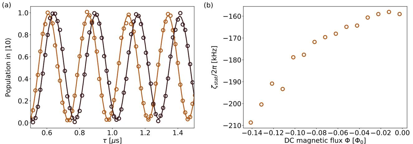
Figure 7. Measurement of the static ZZ-shift: (a) Population in  $|10\rangle$  as a function of the delay time  $\tau$  in the Ramsey-type sequence described in the text, red with dark symbols corresponding to  $U = I$  and bright symbols to  $U = X_{\pi}$ . (b) Measured static ZZ shift  $\zeta_{\text{stat}}$  as function of the DC magnetic flux  $\Phi_{\text{DC}}$ .
