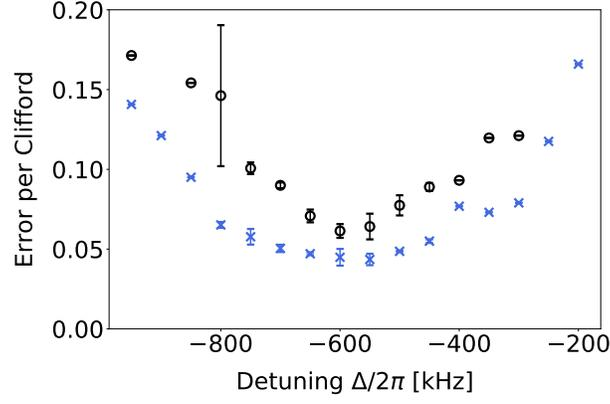
Figure 4. Error per Clifford as a function of the drive detuning  $\Delta$ . Shown are the interleaved (black circles) and the reference (blue crosses) randomized benchmarking curves.
