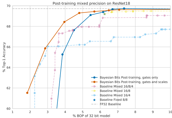
Figure 4. Pareto fronts. Pareto fronts of Bayesian Bits post-training and the baseline method, as well as a fixed (post-training) 8/8 baseline. For our method mean results over 3 runs are plotted with solid lines.
