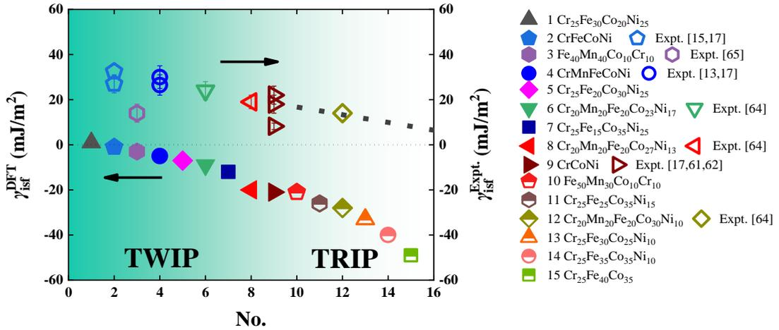
**Figure 3.** Correlation between the calculated SFEs ( $\gamma_{\text{isf}}^{\text{DFT}}$ , filled and half-filled symbols) and the observed strengthening mechanisms (TWIP/TRIP) [61, 64, 109-111] in a group of MEAs and HEAs. Available experimental SFEs ( $\gamma_{\text{isf}}^{\text{Expt.}}$ , empty symbols) are also plotted for comparison. Experimental SFEs for TRIP alloys are usually not available but should approach zero as indicated by the dashed line according to the experimental
