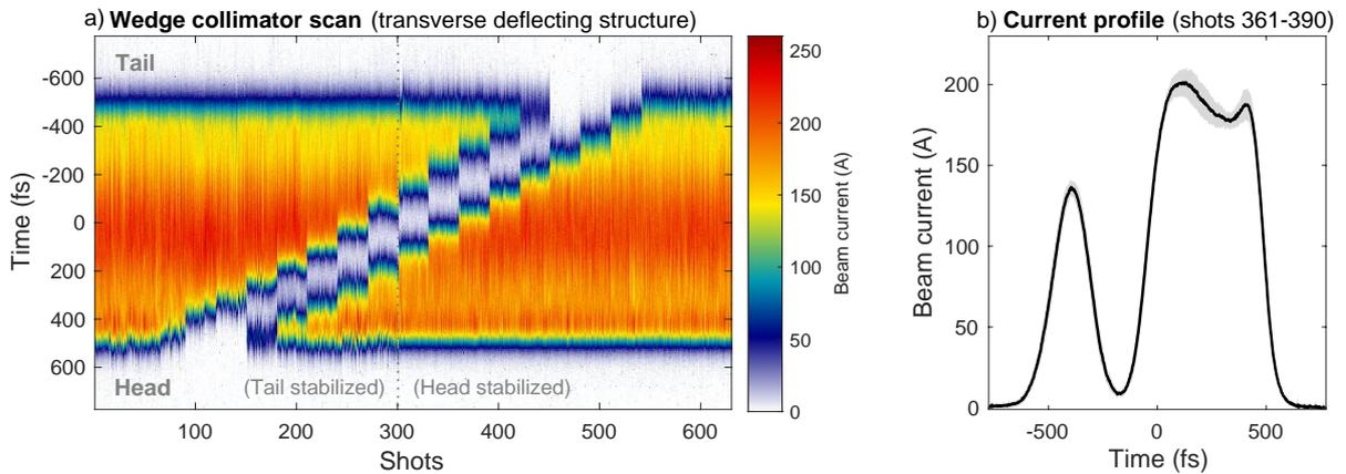
Figure 5: **Two-bunch measurement in a transverse deflecting structure.** Current profile waterfall of horizontal wedge position scan with a moderately compressed beam (a). The single shots are phase corrected with a threshold for the bunch tail (first  $\sim 300$  shots) and then for the bunch head. Mean current profile and its root mean square (gray band) of one particular collimator position (b).
