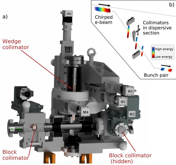
Figure 2: **3D CAD model of the three collimator device.** (a) The block collimators are adjustable in the horizontal plane (M1, M2) and act on the head and tail of the bunch. The wedge determines the bunch separation width (M6) and position (M5). Further alignment of the wedge is available by rotation about the vertical (M4) and the longitudinal (beam) axis (M3). (b) Schematic layout of bunch collimation in dispersive section.
