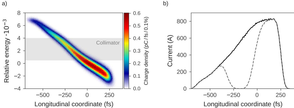
Figure 1: **Two-bunch generation using a collimator in a dispersive section.** The longitudinal phase space is linearised in the FLASH accelerator and measured by a transverse deflecting structure in a photon beamline parallel to FLASHForward (a). A collimator in a dispersive section effectively cuts the original bunch (solid) in a driver–witness bunch pair (dashed) (b).
