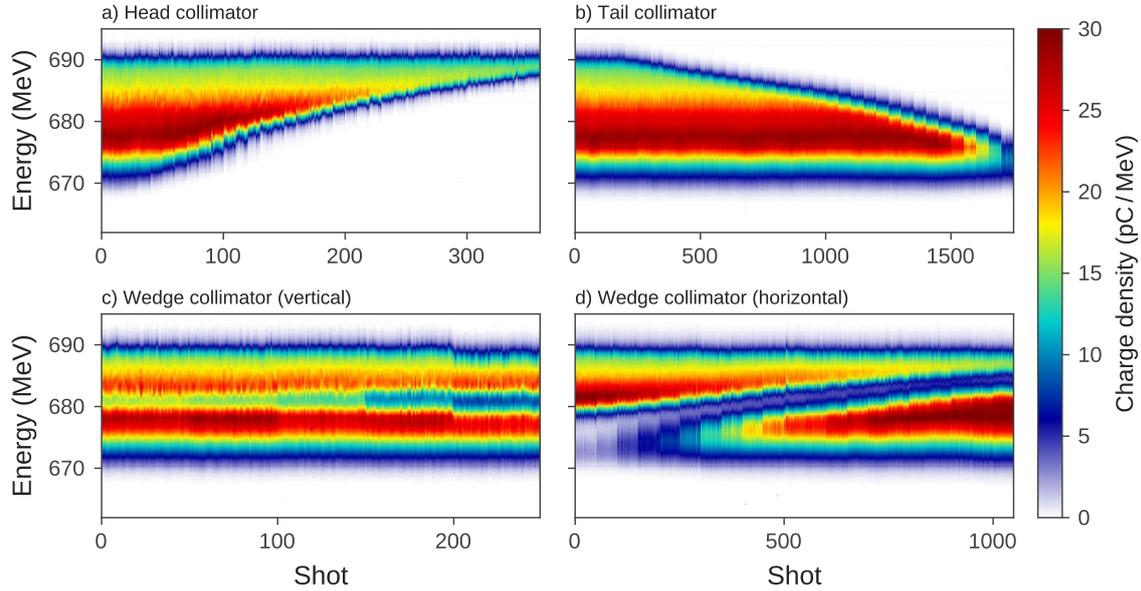
Figure 4: **Energy projection waterfall of collimator position scans.** Two blocks can be used to remove the low-energy head (a) or the high-energy tail (b) of the bunch. Separation width (c) and position (d) is adjusted by a wedge-shaped collimator, which can be positioned in the vertical and horizontal (dispersive) plane.
