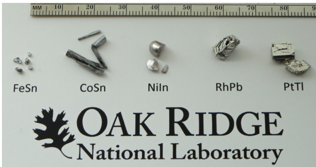
FIG. 2. A photo of the CoSn-type samples with steel scale. The pale-blue metallic luster of CoSn is evident but the pale-pink hue of NiIn doesn't show up well.
