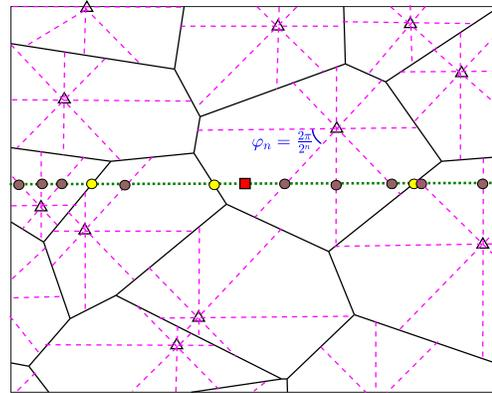
Fig. 1. A snapshot of a Poisson cellular network with directional beamforming to an MT. In this case, each BS has  $2^3 = 8$  beams, i.e.,  $n = 3$ .  $\triangle$  : Base station (BS), red square : MT location, brown filled circle : Beam reselection location, yellow filled circle : BS handover location, solid black lines : Cell boundaries, dashed lines : Beam boundaries, and dotted line : Path of the MT.
