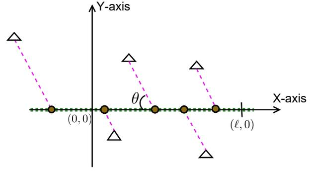
Fig. 5. At most one beam reselection for a BS.  $\triangle$  : Base station (BS), brown filled circle : Beam reselection location, dashed lines : Beam boundaries, and dotted line : Path of MT along the X-axis.
