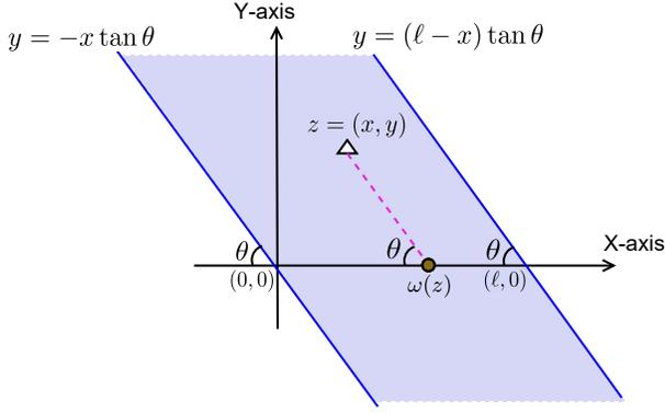
Fig. 6. Strip  $\mathcal{S}$  (shaded area) between two blue solid lines with angle  $\theta$  with the  $X$ -axis.  $\triangle$  : BS, brown filled circle : Beam reselection location, and dashed line : Beam boundary.
