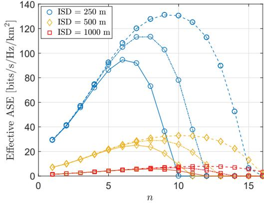
Fig. 2. **FR1**: Effect of average inter-site distance (ISD) on the effective ASE for different  $n$ . Dashed line:  $v = 3$  km/h, Dashed-dotted line:  $v = 30$  km/h, and Solid line:  $v = 120$  km/h.
