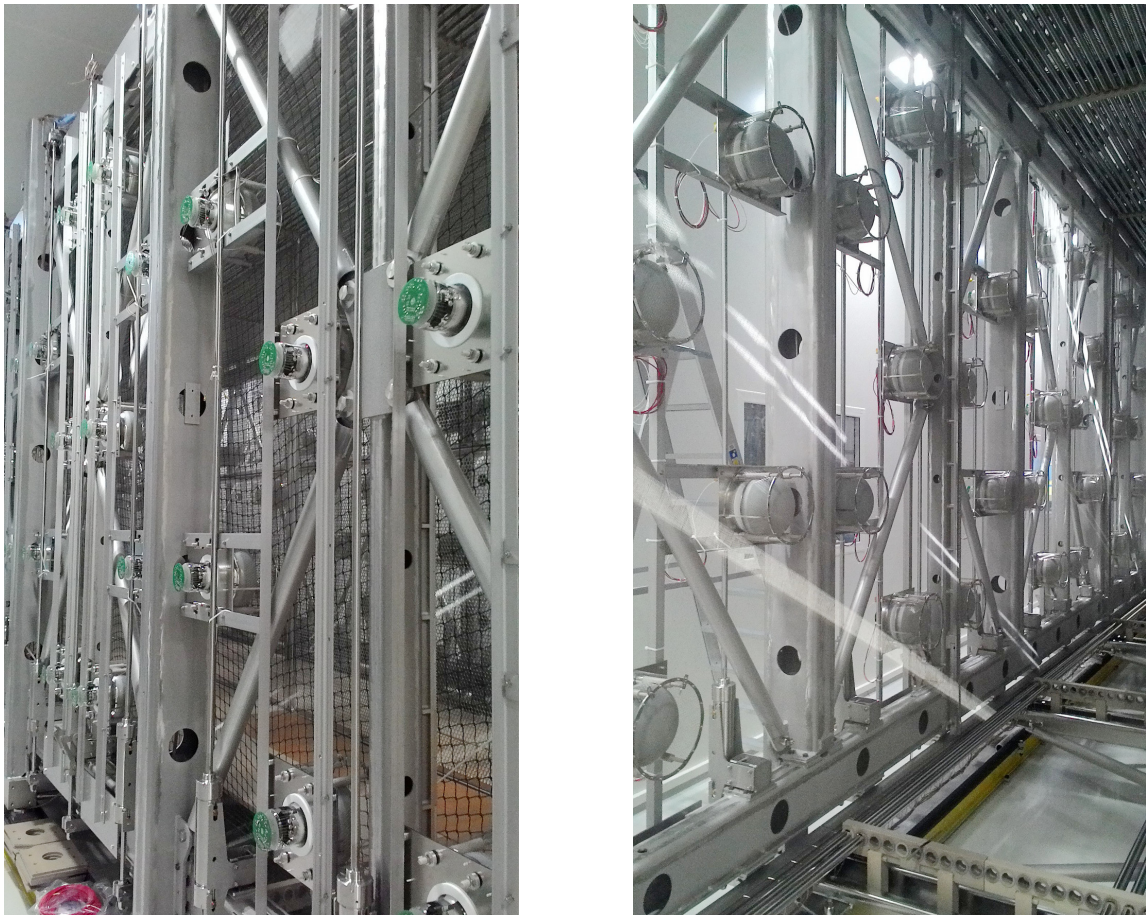
Figure 11. Picture of the PMT supporting system.
