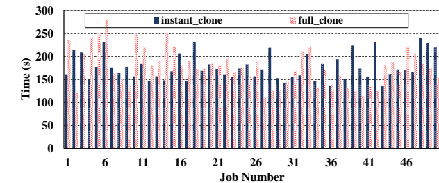
Figure 9: Workload-1: Comparison of Job running time for full and instant clone for 50 jobs.
