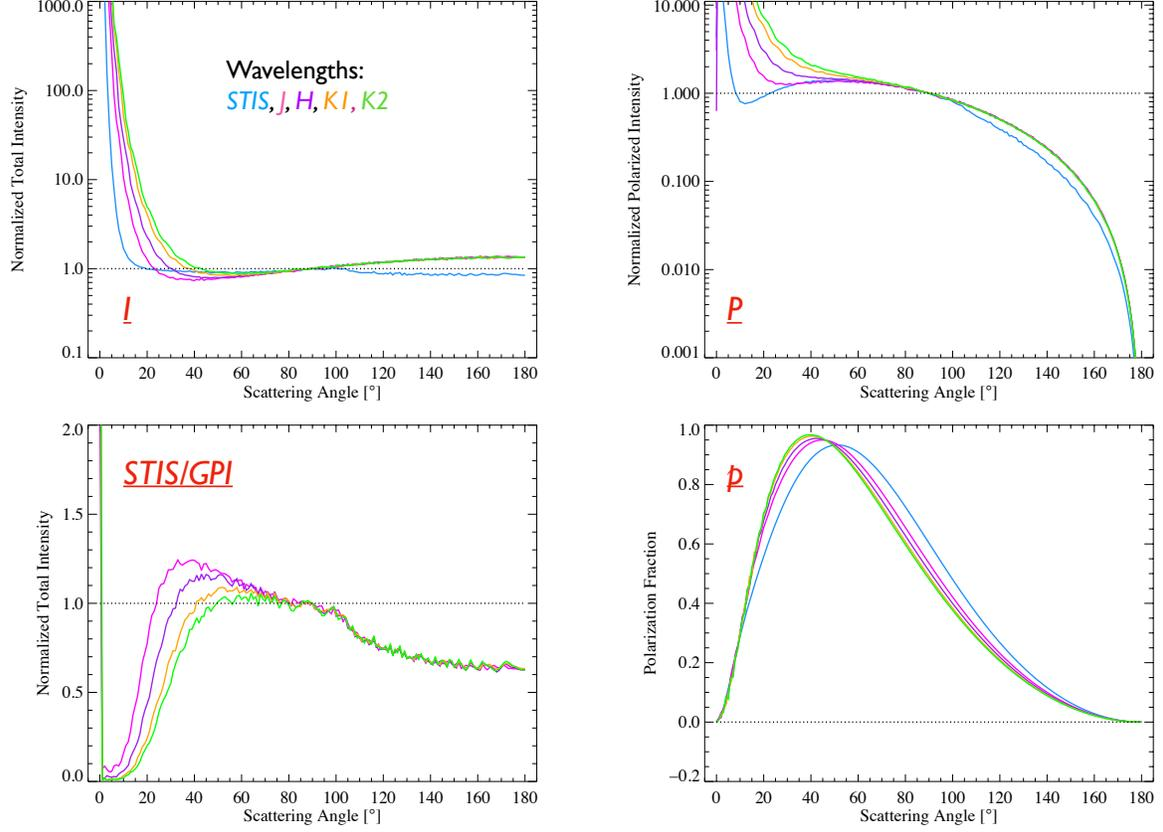
**Figure 17.** (Top-Left) DHS model total intensity scattering phase functions shown for *HST* STIS and GPI J, H, K1, and K2. (Top-Right) DHS model polarized intensity scattering phase functions. (c) (Bottom-Left) Ratio of the *HST* STIS and GPI J, H, and K1 scattering phase functions. (Bottom-Right) The polarization fraction ( $p = P/I$ ) scattering phase functions.
