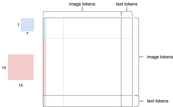
Figure 4. The structure of f(QK^T) in concatenated self-attention, annotated with approximate areas devoted to each ‘type’ of attention (image to image vs. image to text). The blue square represents the 7x7 array of image tokens extracted from block 4 of ResNet; the red square represents the 14x14 array of image tokens extracted from block 3. Each 2d array of tokens is reshaped to a 1d array of tokens by stacking. Finally, the text tokens, shown in green, are added to the bottom.
