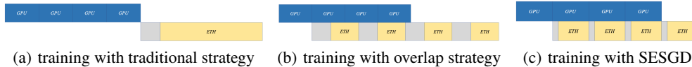
Figure 1: Training with different strategies. A blue block indicates computation time in one layer, which uses the GPU resources. A yellow block corresponds to gradient transmission time in communication, which uses the bandwidth resources. And the grey block presents the idle time during communication, which harms the bandwidth utilization.
