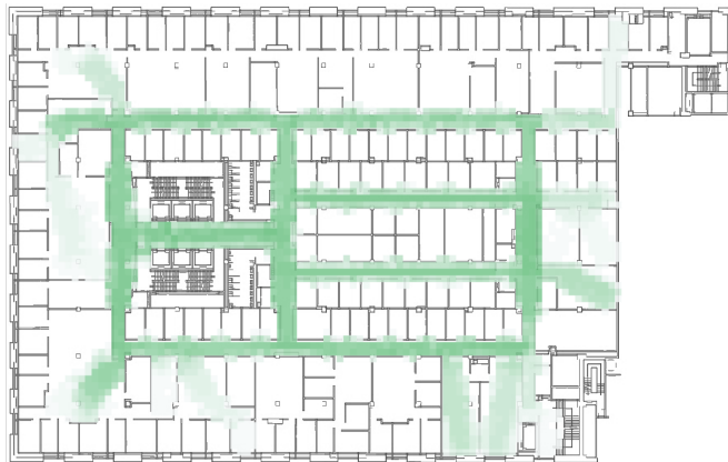
Fig. 6: Average passage coverage over 25 runs in GCWorld. Darker cells were detected more often.
