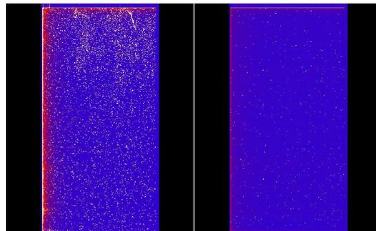
Figure 1: LED-irradiated images with Hitomi (left) and XRISM CCDs (right), which use the same color scale. The bright region indicates light leakages. Note that most of the white dots seen in the XRISM CCD image are of X-ray events from a calibration source <sup>55</sup>Fe. The number of pinholes is given in the text.
