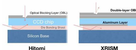
Figure 2: Schematic side views of the Hitomi (left) and XRISM (right) CCDs (not to scale). Expected light paths are drawn as the red arrows.
