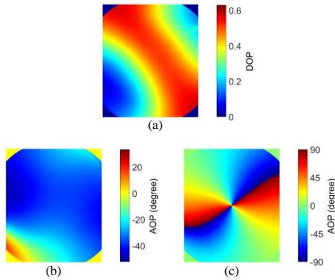
Fig.16 Actual polarization images: (a) DOP image; (b) AOP image; (c) AOPLM image. The four corners of these polarization images cannot be properly imaged due to the short focal lens adopted by the imager, so they are not used in polarized skylight navigation and are set to 0.
