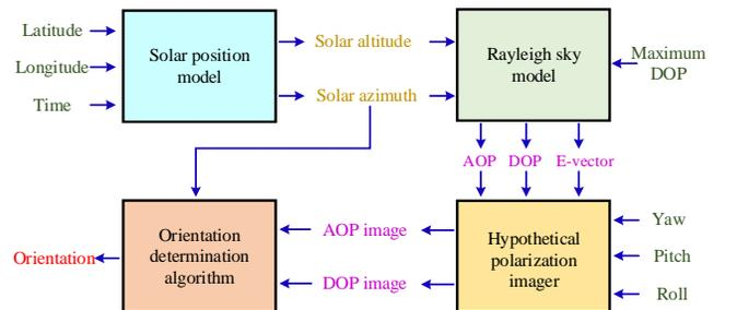
Fig.1 Polarization compass simulation system, where AOP represents the angle of polarization, DOP represents the degree of polarization, E-vector represents the polarization electric field vector. Green words indicate input, the orange words indicate input or process data, pink words indicate process data and red word indicates output.
