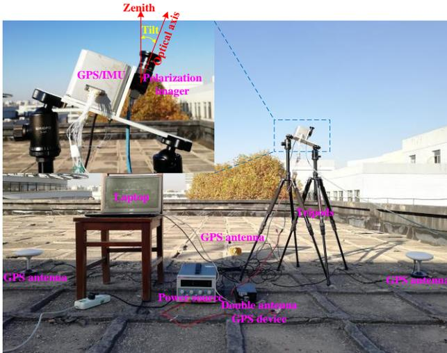
Fig.15 Polarization orientation determination experiment platform.
