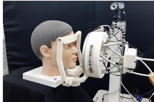
Fig. 6. Autonomous Swab Test Robots [111].
