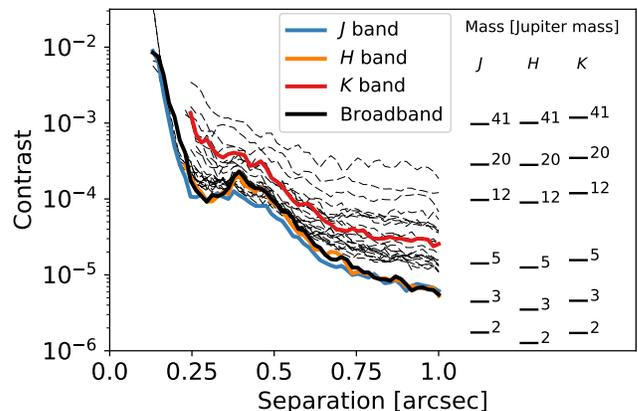
**Figure 6.**  $5\sigma$  contrast limits of our ADI+SDI result. Dashed lines correspond to that at each slice and  $J$ ,  $H$ ,  $K$ , and Broadband ( $JHK$ ) correspond to those of collapsed images at each wavelength, respectively. We also plot mass as a function of contrast at three wavelengths assuming COND03 and 5 Myr.
