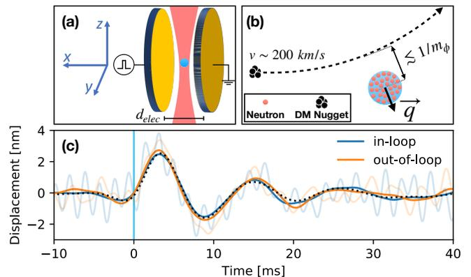
FIG. 1. Schematics of: (a) the levitated sphere and calibration electrodes, and (b) a DM nugget coherently scattering from a sphere via a light mediator, producing a momentum transfer  $\vec{q}$ . (c) Example 4.8 GeV impulse produced by applying a pulsed electric field at  $t = 0$  to a sphere with charge  $-1 e$ . The raw waveform with minimal filtering (light, solid), filtered waveform (dark, solid), and filtered template (dashed) are shown.
