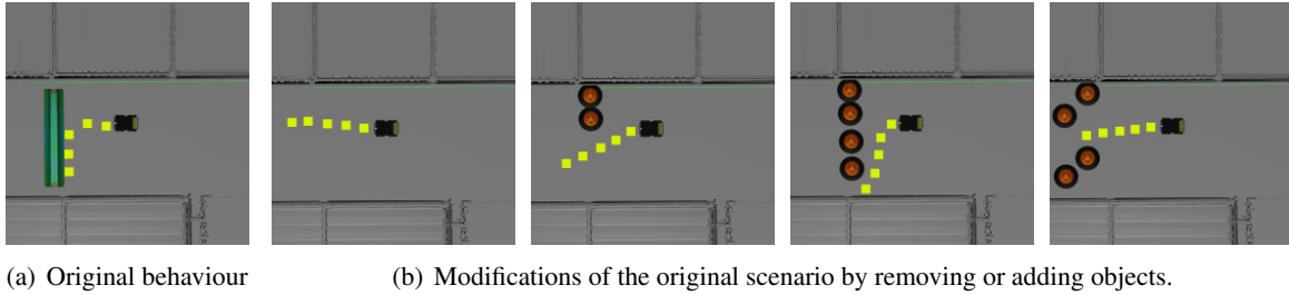
Figure 8: (a) shows the prediction (yellow dots) of the positions for the robot when a green barrier is in front of it. (b) modifications to the original image by removing the barrier or adding new objects in different positions. The new predictions allow the operator to: i) causally infer that the barrier is responsible for the original behaviour, and ii) find a solution for the robot to continue to the goal.
