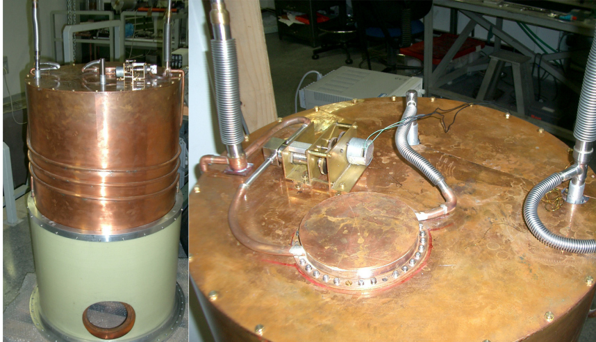
Figure 2: Pictures: on the left the Helium vapor cooled shield, the fiberglass tube support, the serpentine and the exchanger. On the right detail of the exchanger, the valve and the mechanism used to operate the valve, regulating the flux of the vapors.
