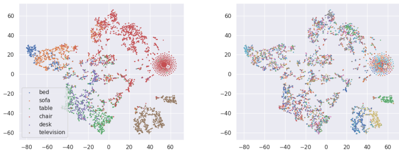
Fig. 8. t-SNE visualization of the object embedding space. Left: We assign the same color to embeddings with the same semantic labels. Right: We assign the same color to embeddings with the same 3D models.
