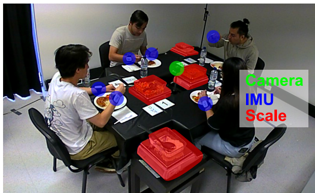
FIGURE 2. Study setup for OREBA-SHA. One camera in the center of the table, IMU on each wrist, and four scales.
