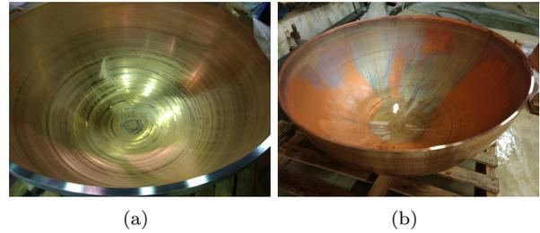
Figure 7: A detector hemisphere following (a) initial cleaning with detergent and (b) chemical etching with an acidified hydrogen peroxide solution. The discolouration observed in the latter is a result of oxidation of the copper and it is removed when the hemisphere is put in contact with the electrolyte.
