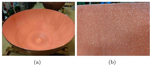
Figure 10: (a) The inner surface of the second hemisphere after electroplating and (b) a close-up of the surface.
