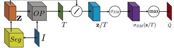
**Figure 3:** Architecture for probability calibration via (local) temperature scaling. The output logit map of a pre-trained semantic segmentation network (Seg) is locally scaled to produce the calibrated probabilities.  $OP$  denotes optimization or prediction via a deep convolutional network to obtain the (local) temperature values. Details of this  $OP$  unit can be found in Appx. B.
