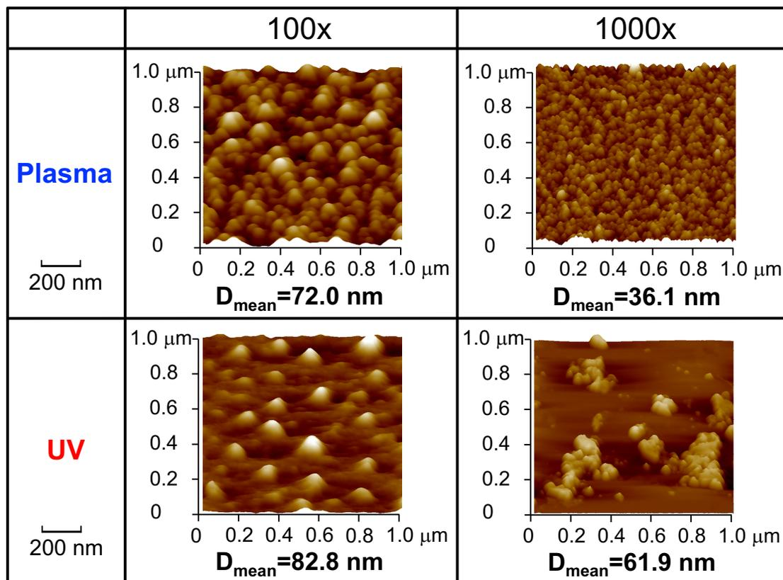
Figure 2. AFM images of particles on the mica substrates in a  $1 \mu\text{m} \times 1 \mu\text{m}$  scanning area for each experiment. The mean diameter ( $D_{\text{mean}}$ , nm) of the haze particles (monomers) is shown under each image.
