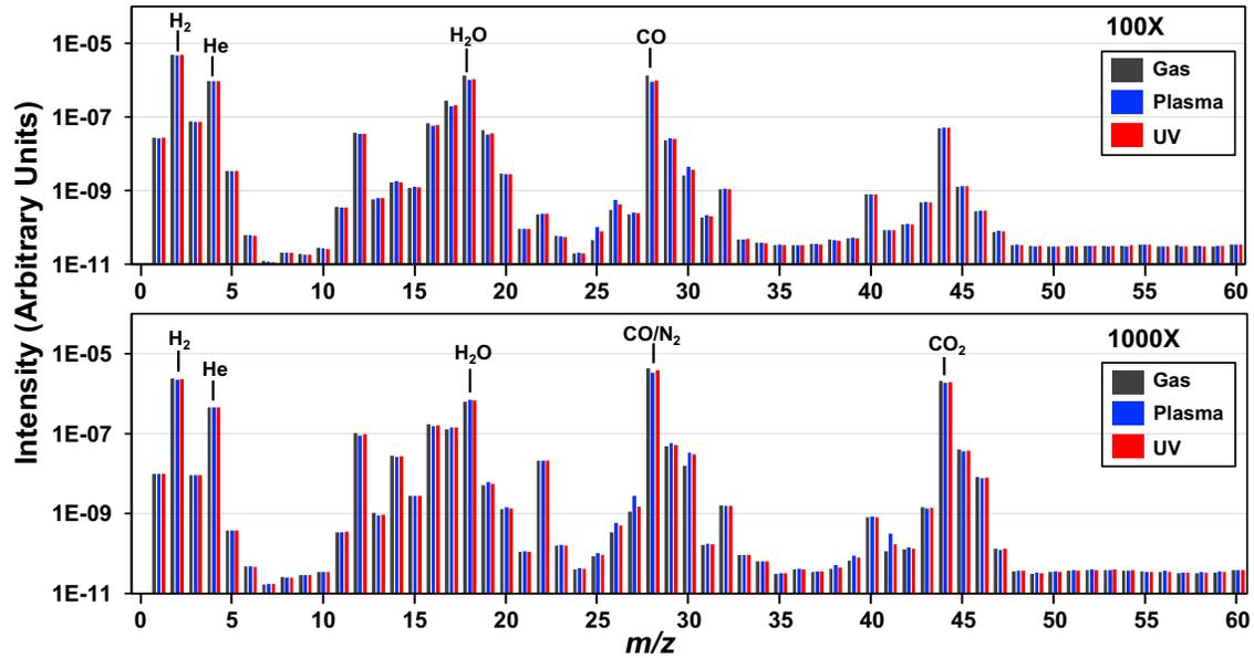
Figure 5. The mass spectra of the gas mixtures in the 100 $\times$  (top) and 1000 $\times$  (bottom) metallicity experiments: initial gas mixture (gray), plasma on (blue), and UV on (red). The initial gas compositions are labeled in the spectra. The decreased peaks indicate the initial gas molecules dissociated under energy exposure while the increased ones are due to the newly formed gas products.
