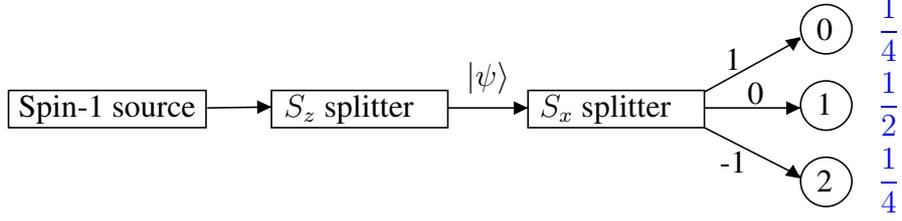
Figure 2: Blueprint for a new QRNG; the values  $\frac{1}{4}, \frac{1}{2}, \frac{1}{4}$  (in blue) correspond to the outcome probabilities of setups prepared in the state  $|\psi\rangle = |\pm 1\rangle$
