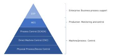
Fig. 1. Automation pyramid (Adapted from: [15]).
