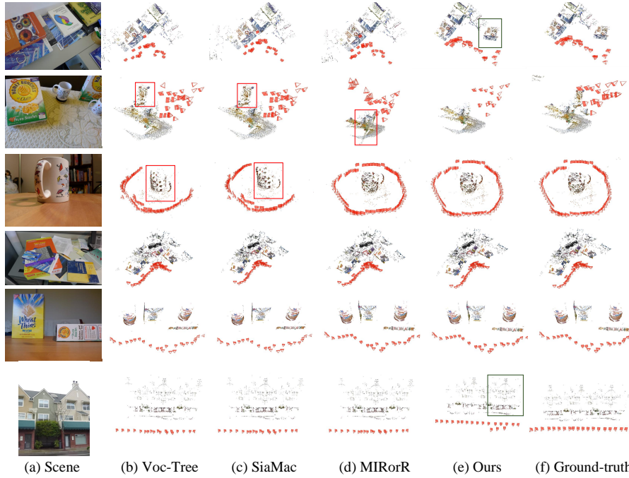
Fig. 6: Experiment results on ambiguous dataset. From top to bottom are Books, Cereal, Cup, Desk, Oats and Street respectively. From left to right: the 1st column - one view of an ambiguous scene, from 2nd to 4th columns - SfM model using matches from Voc-Tree, SiaMAC and MIRorR, the 5th column - SfM model using our retrieved matches, the 6th column - SfM model using manually judged matches. Green box indicates structure only rebuilt by our method, while red box indicates wrong structure reconstructed by comparing methods.
