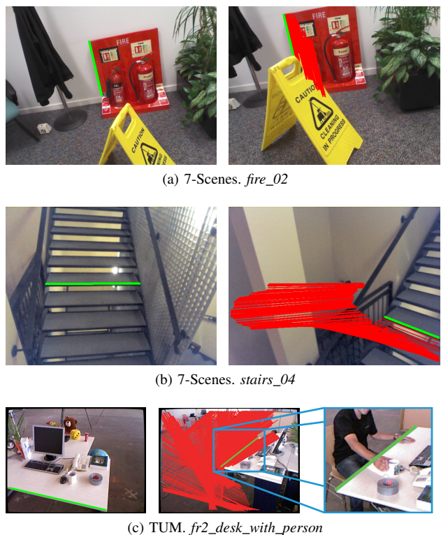
Fig. 11: Line flow results in 3 challenging scenarios: partial occlusion (a), repetitive texture (b), and dynamic object occlusion (c). The left picture of each row shows the first line segment of the line flow (green), while the right one shows the current line segment of the line flow (green) along with previously extracted line segments (red).
