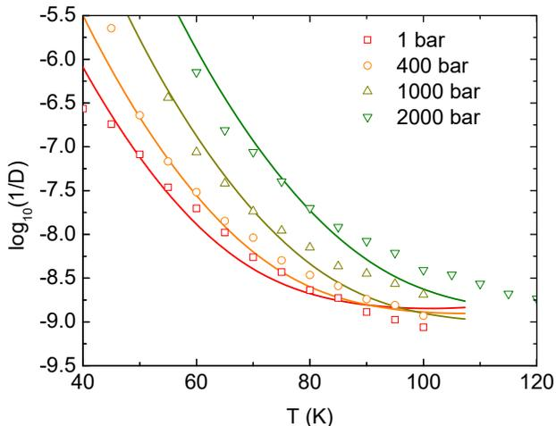
FIG. 3: (Color online) Logarithm of inverse diffusion constant (in unit of  $\text{s}/\text{nm}^2$ ) as a function of temperature at different pressures. Open points are simulations and solid curves correspond to ECNLE calculations.
