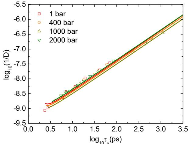
FIG. 4: (Color online) Logarithm of inverse diffusion constant (in unit of  $\text{s}/\text{nm}^2$ ) versus  $\log_{10} \tau_\alpha$  at various pressures. Open points are simulations and solid curves correspond to ECNLE calculations.
