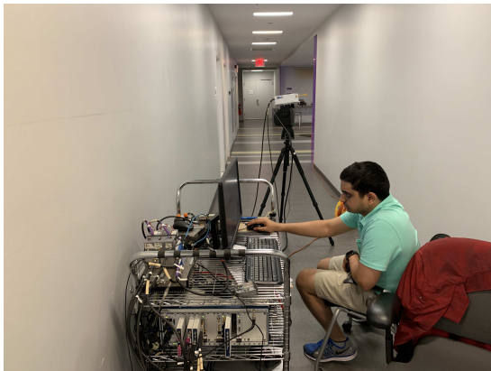
Fig. 7. UE 11 was mounted on a gimbal at a height of 1.5 m in a long corridor.
