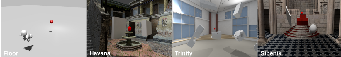
Figure 1: We show the dynamic scenes with various moving objects that are used to evaluate our hybrid sound propagation algorithm. We compute the acoustic scattered fields of each object using a neural network and couple them with interactive ray tracing to generate diffraction and occlusion effects. Our approach can generate plausible acoustic effects in dynamic scenes in a few milliseconds and we demonstrate its benefits for sound rendering in virtual environments.
