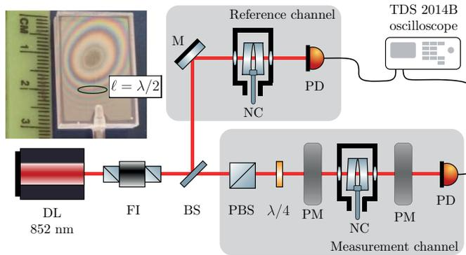
Figure 2: Sketch of the experimental setup. DL — tunable diode laser, FI — Faraday isolator,  $\lambda/4$  — quarter-wave plate, PBS — polarizing beam splitter, NC — nanocell in the oven; PM — permanent magnet, PD — photo-detectors. The reference channel is composed by an auxiliary Cs NC providing a frequency reference at zero magnetic field. The inset on the top left side show a picture of the Cs NC, where the region of thickness  $\ell = \lambda/2$  has been highlighted.
