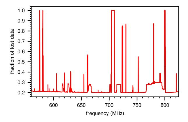
Extended Data Figure 1: The fraction of data excised across the observing band. This includes all data lost due to time-variable effects, including RFI, malfunctioning antennas, power failures, etc. The plotted fraction of lost data was obtained by averaging over the  $\approx 67$  hours of on-source time on the five DEEP2 sub-fields.
