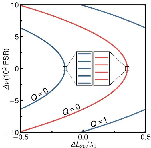
Figure 4. Beat-note frequencies versus cavity length with parity phase shifts. The pump mode is a superposition of  $HG_{20}$  (even) and  $HG_{11}$  (odd), and the considered interactions are  $HG_{20} \rightarrow HG_{10} + HG_{10}$  (blue) and  $HG_{11} \rightarrow HG_{10} + HG_{01}$  (red). The insets show a zoom-in of the degeneracy in each curve, with the horizontal lines indicating the allowed frequencies. The system parameters are the same as in Fig.3.
