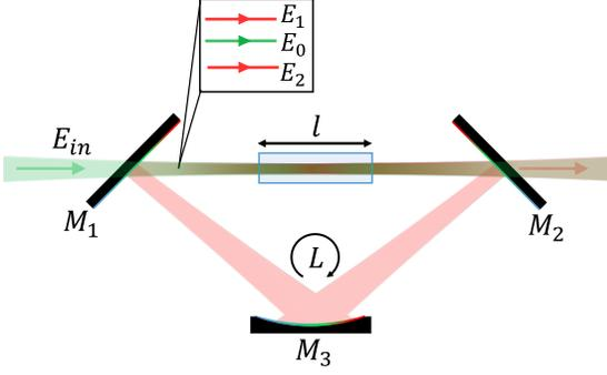
Figure 1. Optical parametric oscillator with a symmetric triangular ring cavity. Mirrors  $M_1$  and  $M_2$  are flat, while  $M_3$  is concave with radius  $R$ . The geometrical length of the round-trip is  $L$ , and the crystal length is  $l$ .
