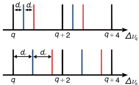
Figure 2. Beat-note frequencies (in units of  $c/L_{eff}$ ) calculated from (25) for  $\delta S = 0$  (black),  $\delta S = 1$  (blue) and  $\delta S = 2$  (red), for a fixed parity of the longitudinal index  $q$ . For the cavity lengths, we considered  $\bar{D}/2R = 0.4$  (top) and  $\bar{D}/2R = 0.9$  (bottom). The shift  $d_\nu$  between adjacent combs is given by (29).
