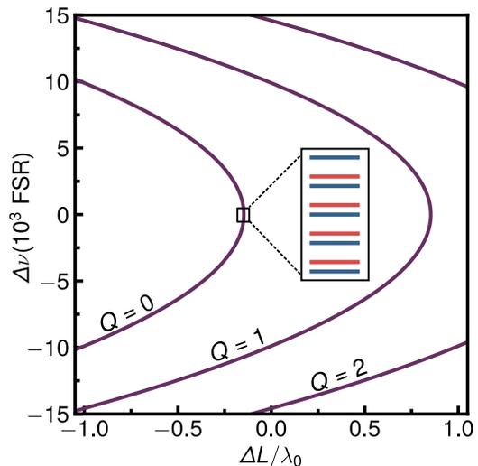
Figure 3. Beat-note frequencies versus cavity length in a type-I OPO. The considered downconverted modes are  $\{S_1, S_2\} = \{1, 1\}$  (blue) and  $\{2, 0\}$  (red), with a second order pump mode  $S_0 = 2$ . The inset shows a zoom-in of the degeneracy, with the horizontal lines indicating the allowed frequencies. The crystal parameters are the same as in Appendix A, and the cavity length is such that  $D/2R \approx 0.75$ .
