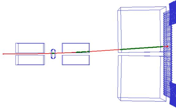
Figure 8.: Top view of a selected event - a single track going through GTPC, VTPC-2 and MTPC-L. The green markers, 125 in total, represent the measured points along the track. The red line is the reconstructed particle trajectory starting from the target on the left to the ToF-F wall on the right. The track's reconstructed momentum is  $p = 30.34$  GeV/c.
