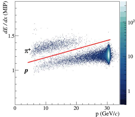
Figure 5.: Distribution of energy loss in the TPCs as a function of momentum. Good separation between  $\pi^+$  and protons is observed. The red line shows the graphical cut applied in the track selection.
