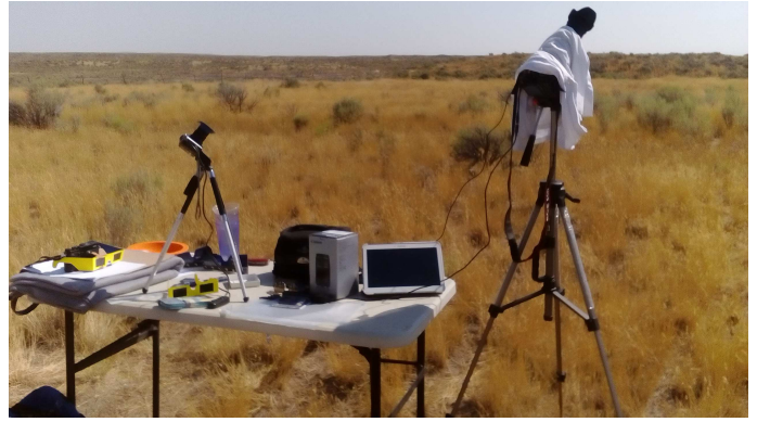
Figure 1. A picture showing the equipment employed on August 21st, 2017 to acquire the TSE observations analyzed here (see text); the picture shows the DSLR camera mounted on the tripod, connected with remote controllers, and covered by a white tissue to reduce as more as possible the overheating by solar illumination during PSE.
