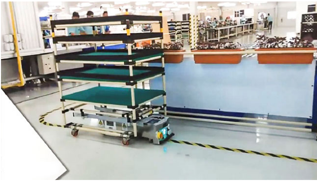
Figure 1: An Autonomous Guided Vehicle (AGV) following a path laid out in tape
