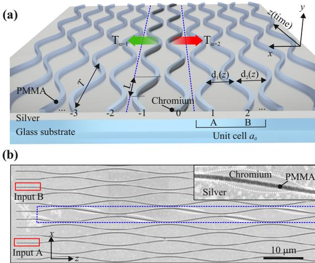
FIG. 4. (a) Sketch of a plasmonic waveguide array featuring unidirectional transmittance. Green and red arrows indicate the low and high loss directions, respectively. (b) SEM scan of a typical sample. Inputs A and B are marked by red boxes and blue dotted line highlight the region with periodic dissipation. The chromium stripe used to implement losses is magnified in the top right corner.
