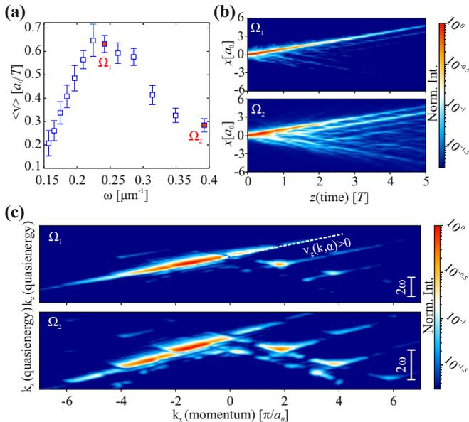
FIG. 5. (a) Measured mean group velocity of a wavepacket versus driving frequency  $\omega$  for the single-site excitation at the input A. (b) Real-space SPP intensity distributions corresponding to the arrays modulated with frequency  $\Omega_1 = 0.23 \mu\text{m}^{-1}$  and  $\Omega_2 = 0.39 \mu\text{m}^{-1}$ . (c) Fourier-space SPP intensity distributions for the same arrays as in (b).
