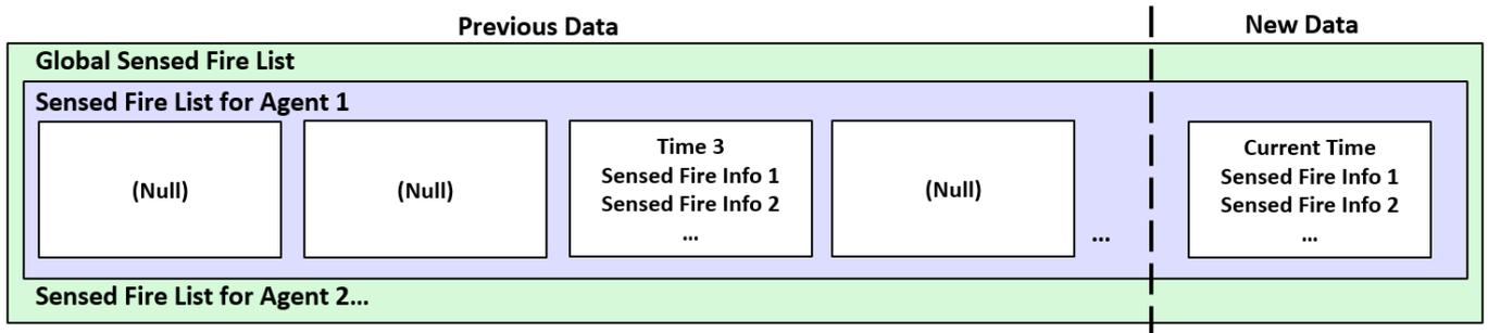
Figure 36: The Structure of the Sensed and Pruned Fire List.
