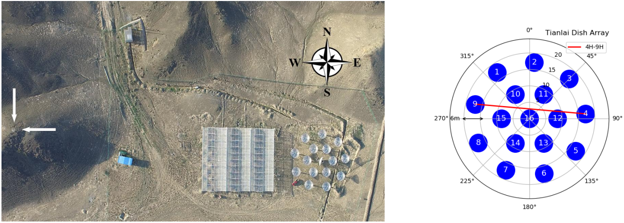
Figure 1. Left: Top view of the Tianlai Dish Array Pathfinder and Cylinder Array Pathfinder taken with a DJI M600 Pro drone at a height of 280 m above the ground. The position of the calibration CNS is indicated by the white arrows on the left. The relative distance vector from the feed in dish 16 at the center of the array (when pointed toward the zenith) to the CNS is [-184.656, 13.915, 12.588] meters, with x,y,z to the east, north, and zenith. The CNS is in the far-field of all dishes in the dish array. Right: A schematic diagram of the Tianlai Dish Array; 0^\circ coincides with North.
