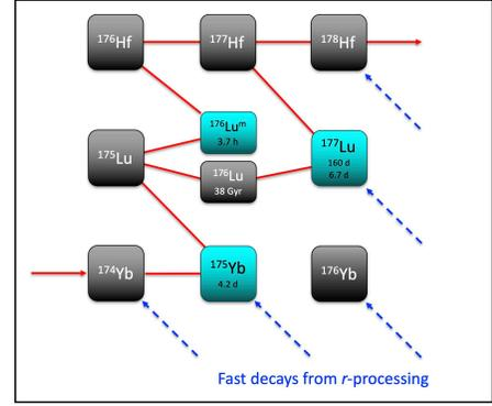
**Figure 15.** The neutron-capture path around  $^{176}\text{Lu}$  and  $^{176}\text{Hf}$  in the chart of the nuclei, when the isomeric state and the ground state of  $^{176}\text{Lu}$  are not thermalized. See text for comments.
